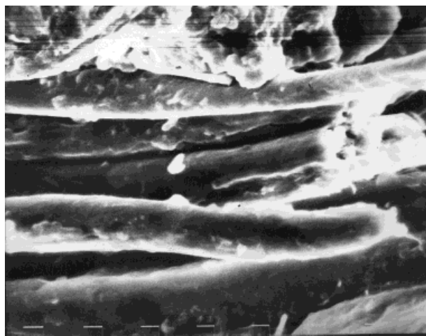
Figure 11 SEM of untreated bagasse composite pressed at 170°C for 8 min.
